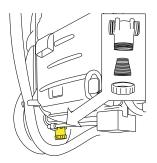
Check the dirty water tank float is undamaged and clean and moves freely on the pin.
