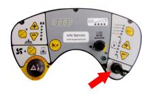
Press the brush button to enable brush and suction motor operation.
