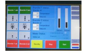
To stop working with Hot water, press the burner off, and the heating-unit will stop.
