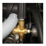
WARNING! The maximum working pressure is 90 bar.
