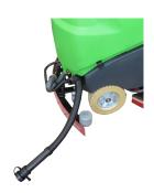
Clean the dirty water tank with water or water and detergent.
