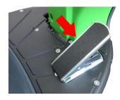
If necessary, release the service or parking brake.
