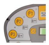
The machine can be operated without using the 3 cleaning programmes provided by the manufacturer. In this case, the brush and suction motors must be turned on and the quantity of detergent regulated manually by pressing the buttons shown.
