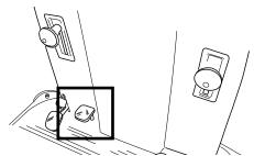
To stop the machine, press the brake pedal, which also acts as parking brake, using the special locking lever.
