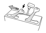
Press the accelerator pedal to start travel, pressing it to the right the machine will move forwards, pressing it to the left the machine will move backwards.
