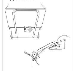
Check and remove any debris wrapped around the side brushes and on the centre brush.
