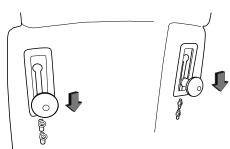
Activate suction using the lever, adjusting air flow to ensure suction of the dust Do not use suction on wet surfaces.
