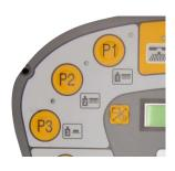
The machine can be operated without using the 3 cleaning programmes provided by the manufacturer. In this case, the brush and suction motors must be turned on and the quantity of detergent regulated manually by pressing the buttons shown.
