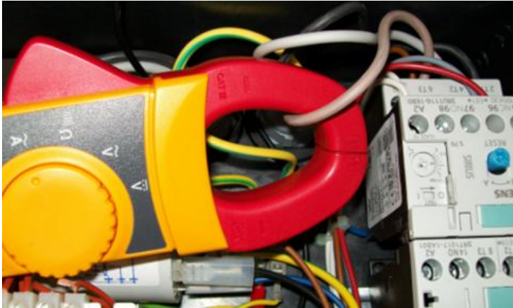
Check the Amperage with a Amp clamp meter
