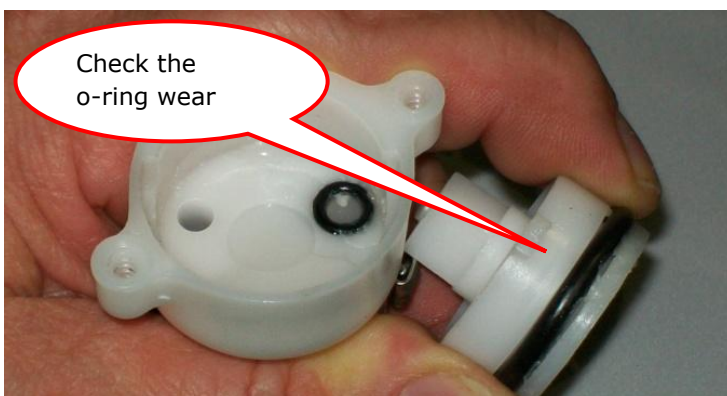
O-ring of detergent tap in detail
