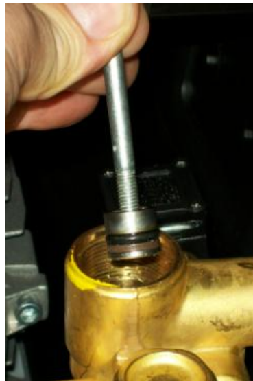
Remove the by-pass seat, use a M6 screw
