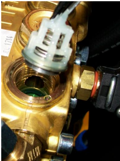
Strip out the valves
