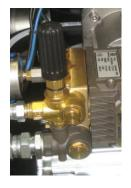
**WARNING!** The maximum working pressure is 50 bar.
