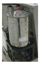
The powerunit is completed built on a frame, together with the fuel tank, installed in a completely covered foolding hood with gas springs, which can be opened/closed.
